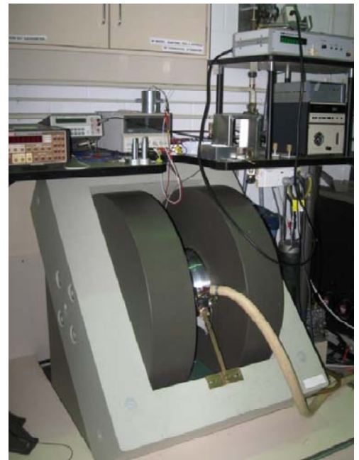
System for conventional and pulsed ESR (4.2 - 300 K, 0 - 1.6 T)
